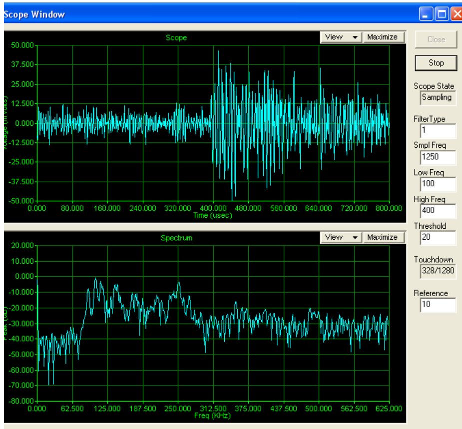
Figure 10: AE signal in time domain and frequency domain during initial touchdown
