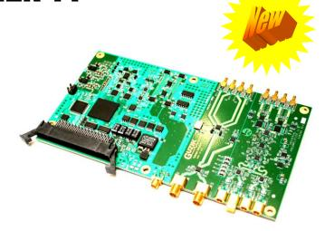
Universal Preamplifier 11 (UP11) is designed for new generation high data rate front end headamplifier and 2011 Headloader. With new Guzik RWA-4000 series UP11 allows to achieve the maximum write data rate 8 Gbit/sec. The bandwidth of read channel extends from DC to 3.2 GHz and allows for reading the perpendicular recording signals without losing DC components. UP11 is compatible with previous generation of Guzik RWA-2000 series.
