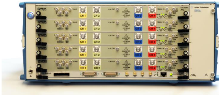
20 channels of 10 GSa/s in the Keysight M9505A 5-slot chassis
