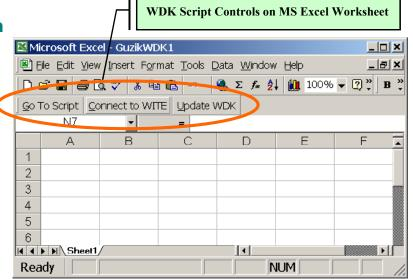
The new script version of Guzik WITE32 Development Kit (WDK32) allows for interactive execution of all Guzik WDK32 functions including RWA and spinstand control functions, measurement functions, and operations. The WDK Script is based on the Microsoft Visual Basic for Applications (VBA) engine and is integrated into Microsoft Excel.
