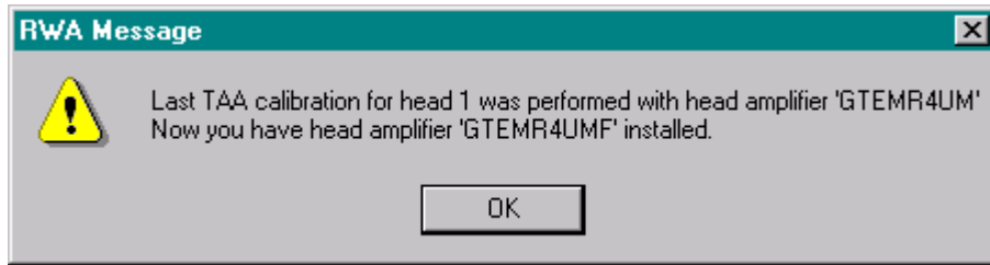
Figure 2: RWA Message, TAA Calibration for Different Head Amplifier Model or Head Amplifier ID
