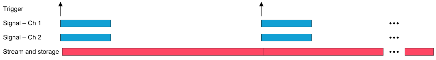
Figure 11. Segmented streaming of two channels with 10 GS/s sampling rate
