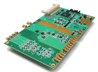
The Universal Preamplifier 8 (UP8) is specially designed for operation with the new RWA 2000 series and can achieve a maximum data rate only with the 2002, 2003, and 2004 models. At the same time, it can be used with our previous generation of test equipment such as the RWA2585.
